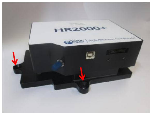
Figure 29 a) and b). Unplugging the USB connector and b) spectrometer baseplate assembly
