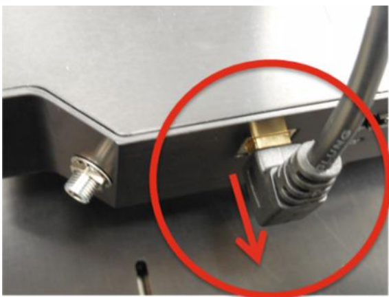
Figure 29 a) and b). Unplugging the USB connector and b) spectrometer baseplate assembly
